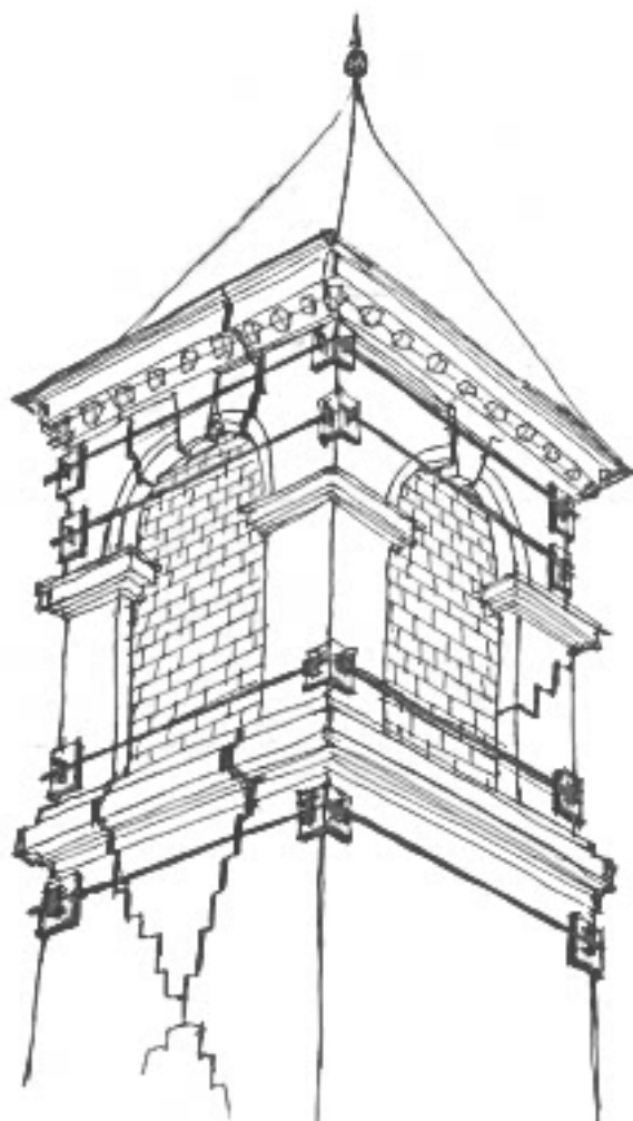
Walling up of openings and strapping
