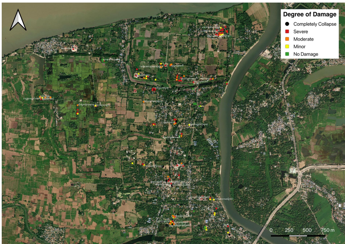
Map Showing the Extent of Damage, Inwa
